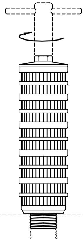
1. Nozzles have to be stored free from frost, do not install at temperatures below 0° C!
